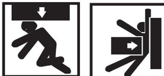
**Heavy loads can crush. Do not allow any body parts to come under the tank cover or between the tank cover and a stationary object. Death or serious injury can result.**
