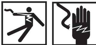
Take great care when working around energized electrical equipment. Contact between unprotected body parts and electrical conductors can cause serious injury or death. Do not wear jewelry or other conductive items while servicing energized electrical equipment. Failure to comply with these precautions can cause serious injury or death.
