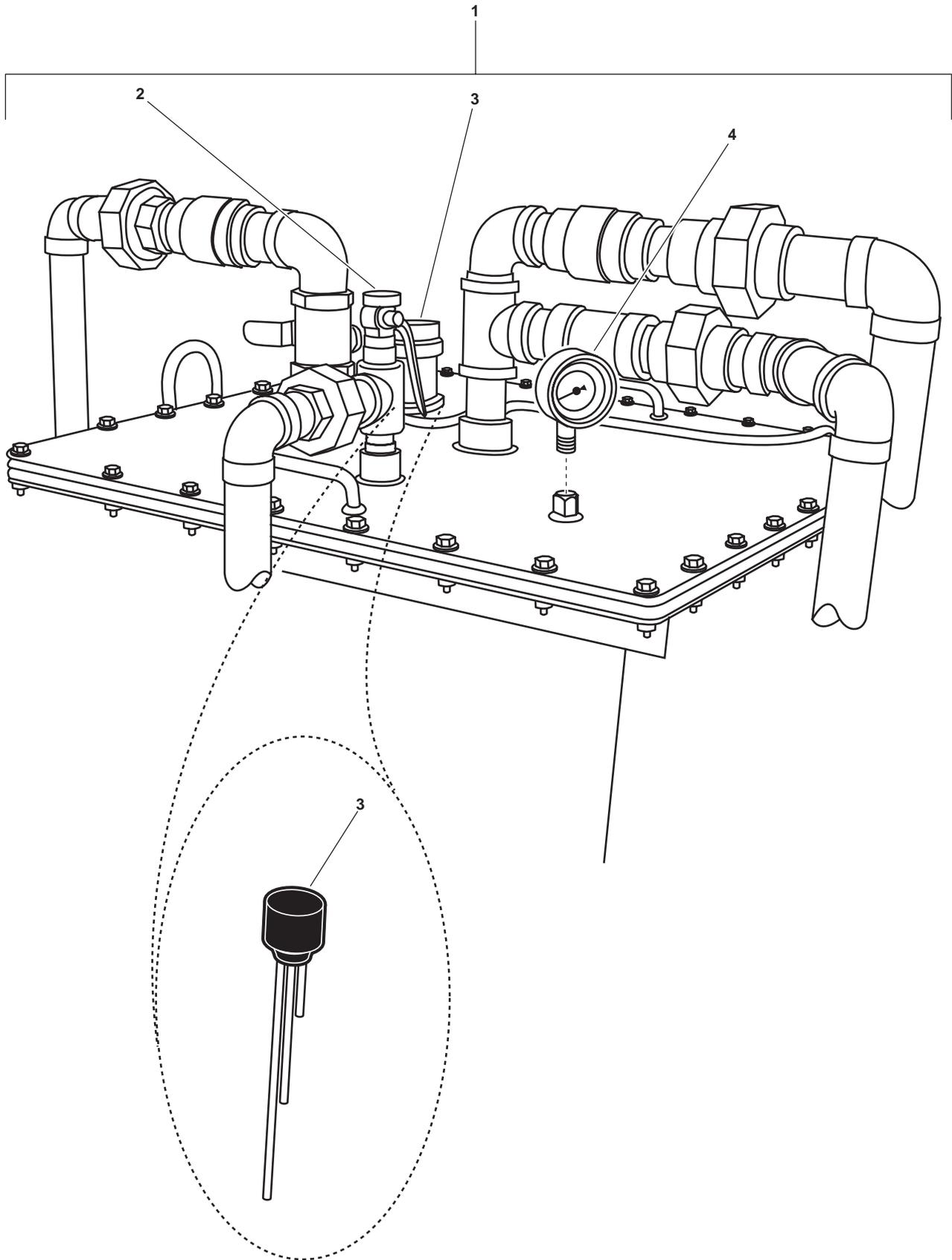
Figure 1. Oil Water Separator (Sheet 1 of 8)
