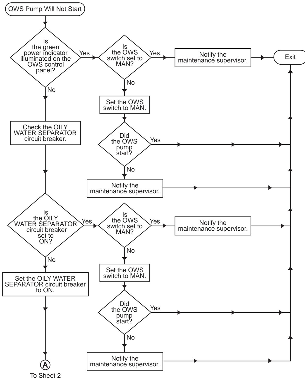
Procedure 4. OWS Pump Will Not Start (Sheet 1 of 2)
