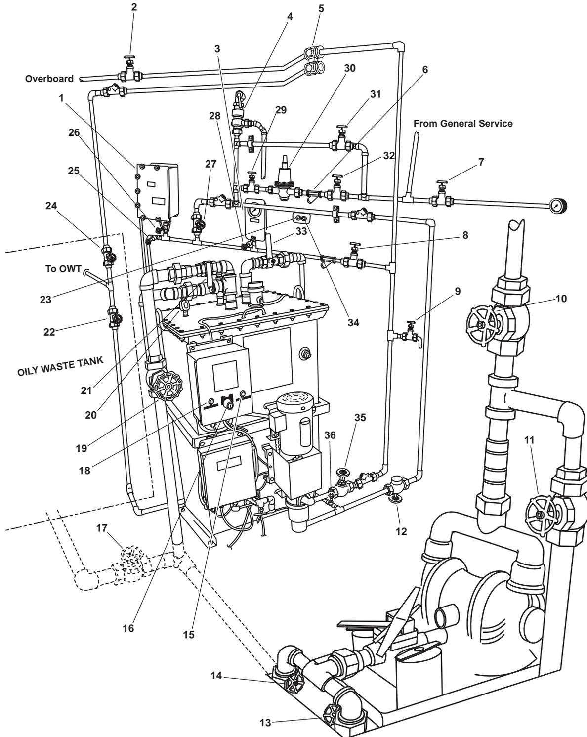
**Figure 1. Oil Water Separator (OWS) and Oil Content Monitor (OCM), Engine Room**
