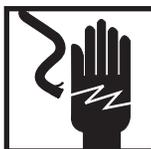
**ELECTRICAL** - electrical wire to hand with electricity symbol running through hand shows that shock hazard is present.
