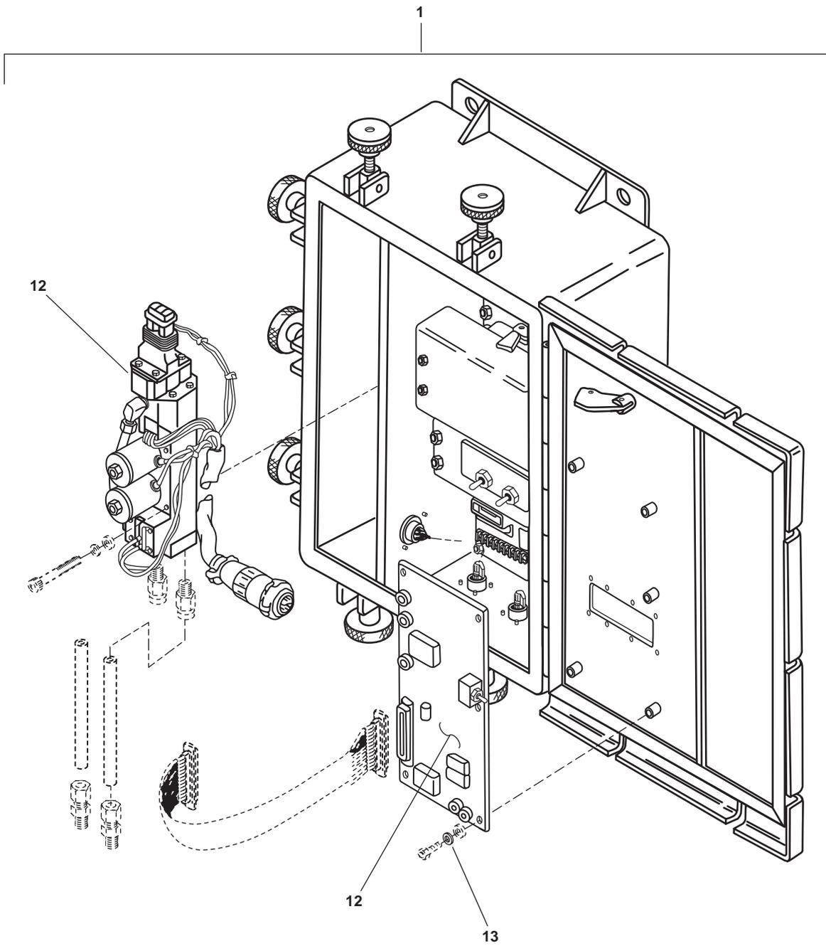
Figure 2. Oil Content Monitor (Sheet 3 of 6)
