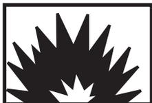
**EXPLOSION** - rapidly expanding symbol shows that the material may explode if subjected to high temperatures, sources of ignition, or high pressure.
