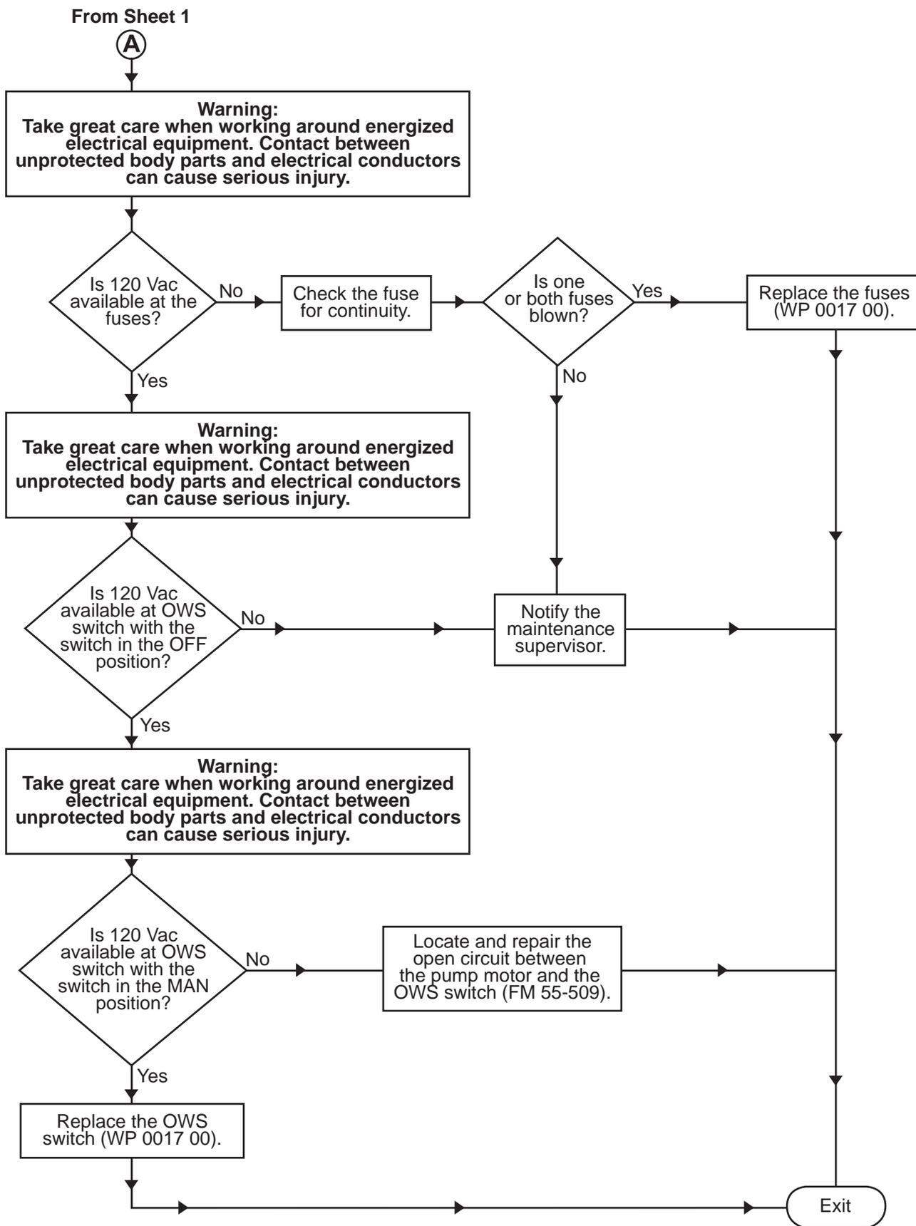
Procedure 7. OWS Fails To Operate In MAN Mode (Sheet 2 of 2)
