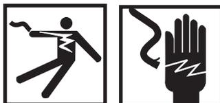
**Death or serious injury can result from contact with live electrical circuits. Before beginning work on this, or any other electrical circuit or equipment, make certain electrical power is OFF, locked out, and tagged out IAW FM-55-502.**
