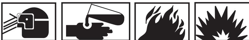
Do not allow hydraulic fluid, engine oil, or cleaning solvents to come in contact with unprotected skin or eyes. Prolonged skin contact can cause illness or injury. Eye contact can cause serious injury. Always wear chemical protective gloves and goggles when handling hydraulic fluid, engine oil, and cleaning solvents. Failure to follow these precautions can result in illness or serious injury.
