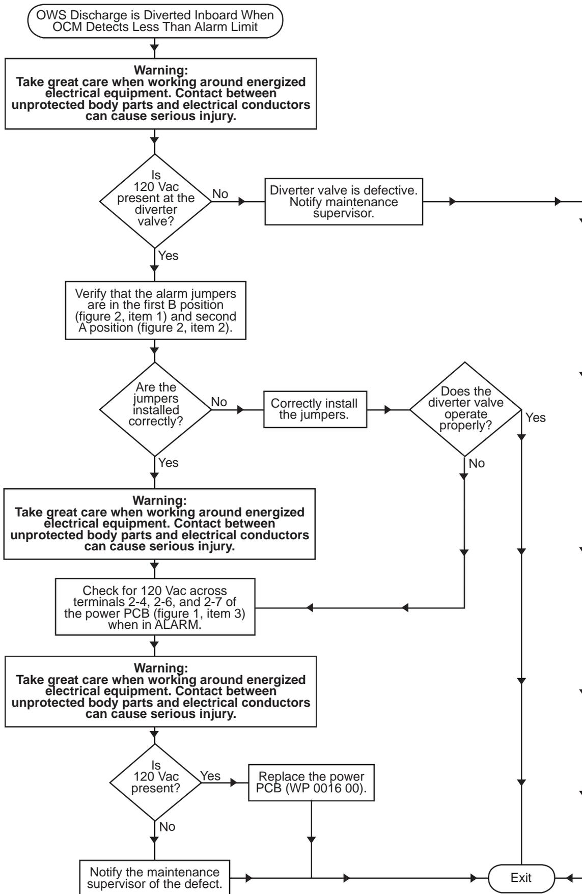
Procedure 17. OWS Discharge Is Diverted Inboard When OCM Detects Less Than Alarm Limit
