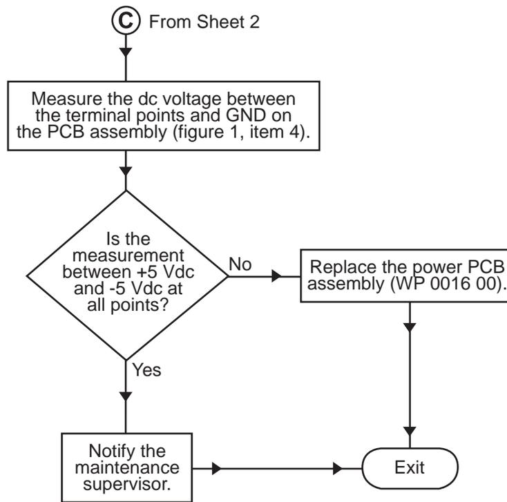
**Procedure 11. OCM POWER ON Indicator Does Not Light (Sheet 3 of 3)**
