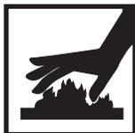
**HOT AREA** - hand over object radiating heat shows that part is hot and can burn.
