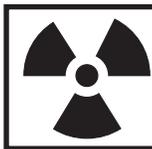
**RADIATION** - three circular wedges show that the material emits radioactive energy and can injure human tissue.
