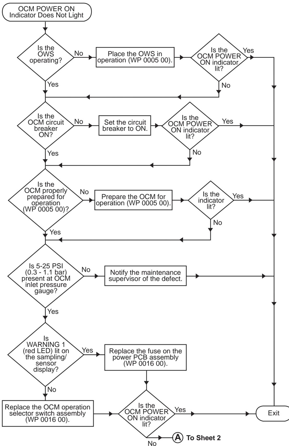
Procedure 11. OCM POWER ON Indicator Does Not Light (Sheet 1 of 3)
