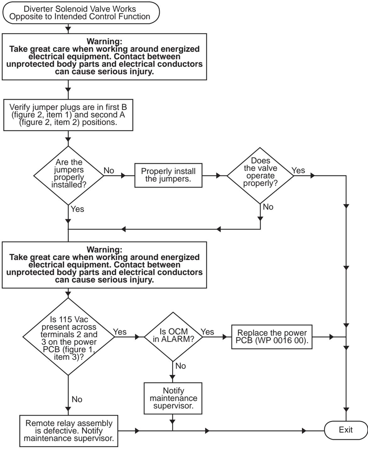
Procedure 21. Diverter Solenoid Valve Works Opposite To Intended Control Function
