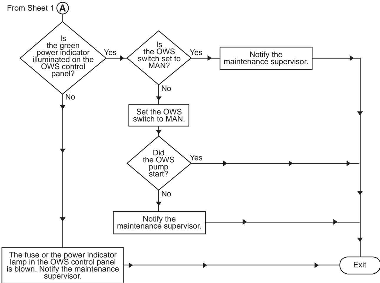
Procedure 4. OWS Pump Will Not Start (Sheet 2 of 2)
