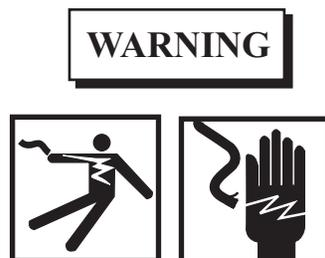
**Take great care when working around energized electrical equipment. Contact between unprotected body parts and electrical conductors can cause serious injury or death. Do not wear jewelry or other conductive items while servicing energized electrical equipment. Failure to comply with these precautions can cause serious injury or death.**
