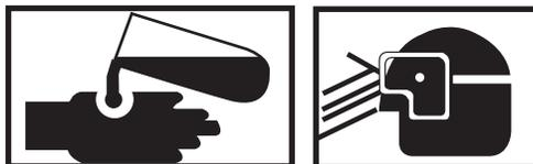
**Do not allow oily water to come in contact with unprotected skin or eyes. Prolonged skin contact can cause illness or injury. Eye contact can cause serious injury. Always wear chemical protective gloves and goggles when handling oily water. Failure to follow these precautions can result in illness or serious injury.**
