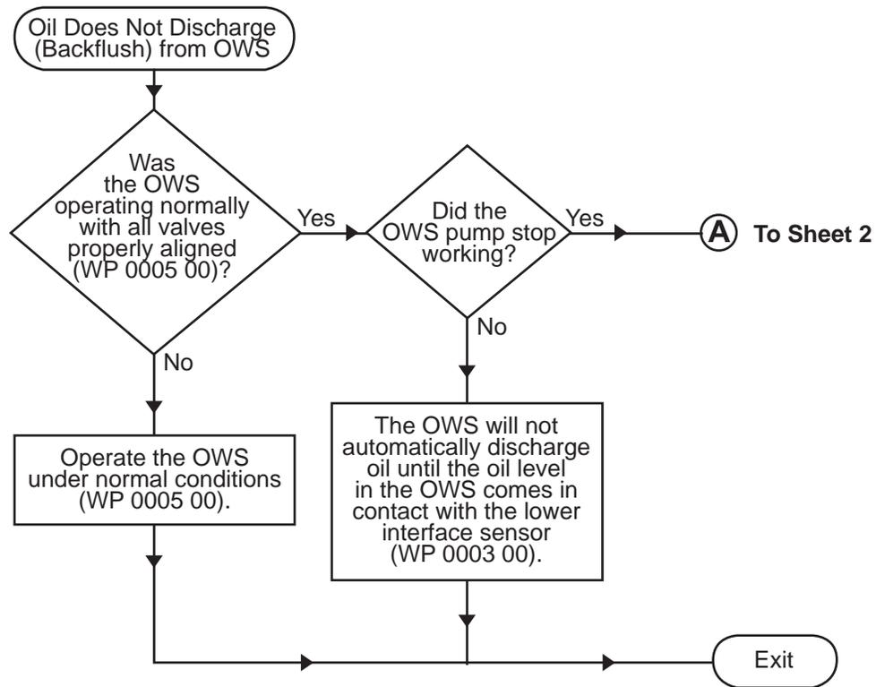
Procedure 9. Oil Does Not Discharge (Backflush) From OWS (Sheet 1 of 2)
