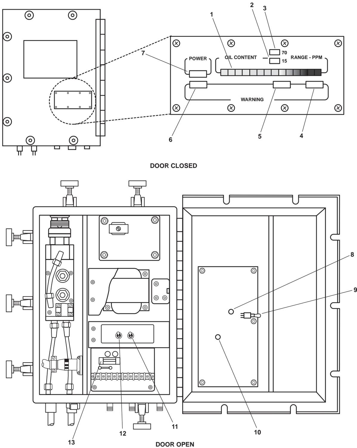
Figure 2. OCM Sampling/Sensor Assembly
