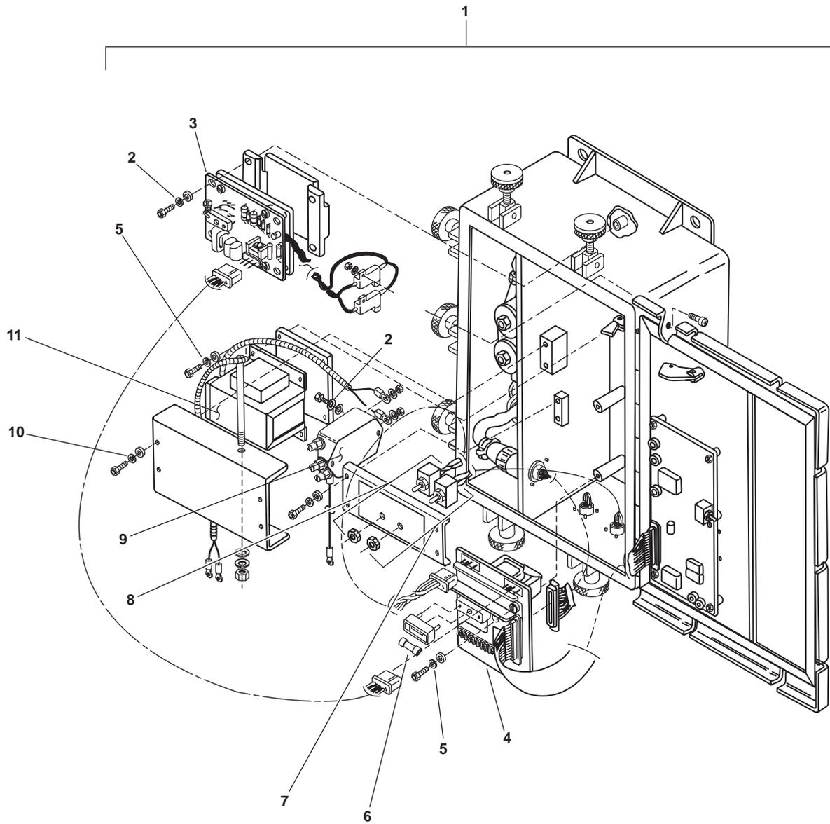
Figure 2. Oil Content Monitor (Sheet 2 of 6)
