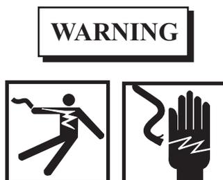
**Take great care when working around energized electrical equipment. Contact between unprotected body parts and electrical conductors can cause serious injury or death. Do not wear jewelry or other conductive items while servicing energized electrical equipment. Failure to comply with these precautions can cause serious injury or death.**
