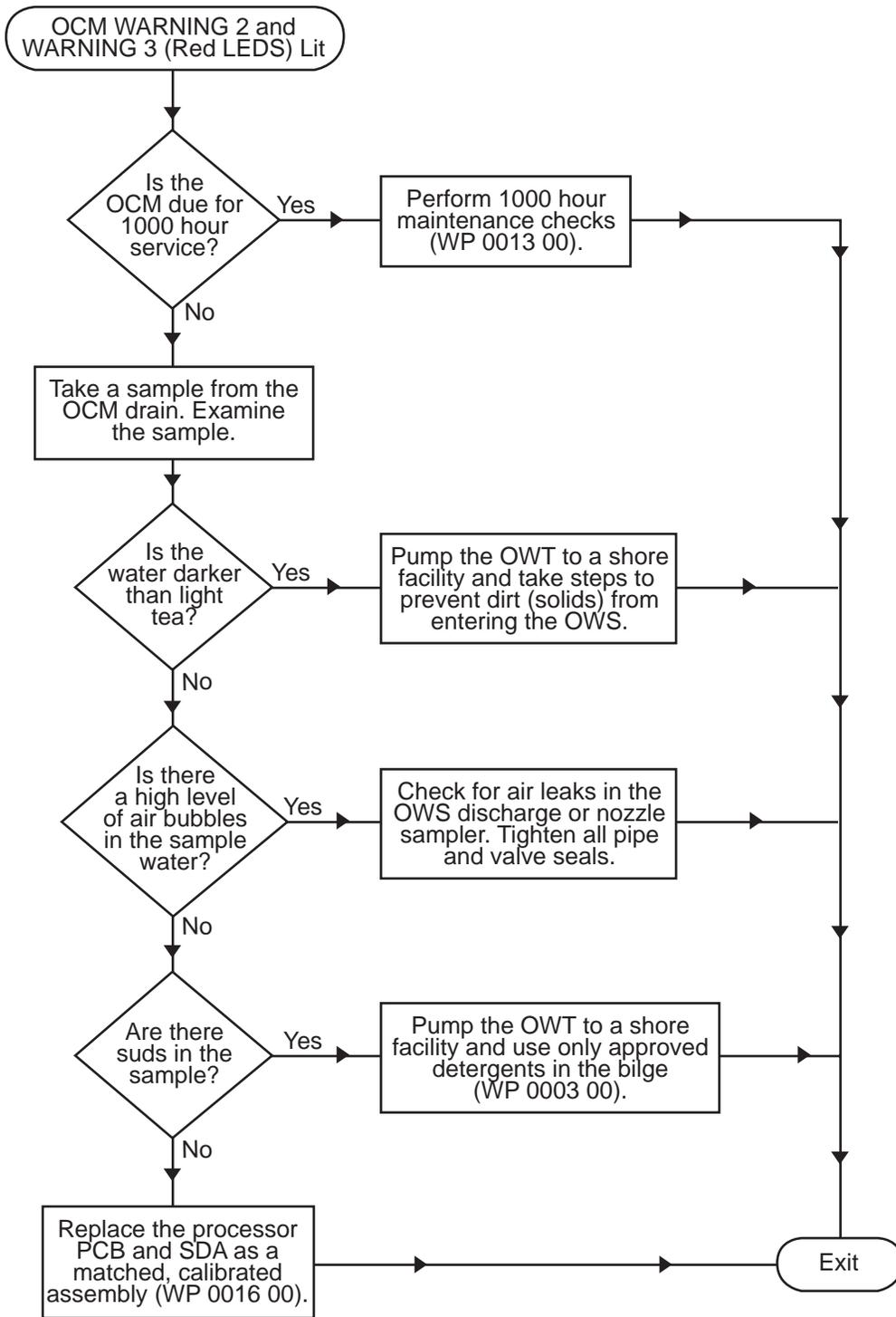
Procedure 15. OCM WARNING 2 And WARNING 3 (Red LEDs) Lit
