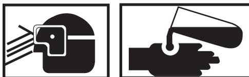
**Removing components by means of wire brushing produces flying particles. These particles can cause serious injury to personnel. Protective goggles, gloves, and long sleeves must be worn at all times during wire brushing operations. Failure to comply can result in serious injury to personnel.**
