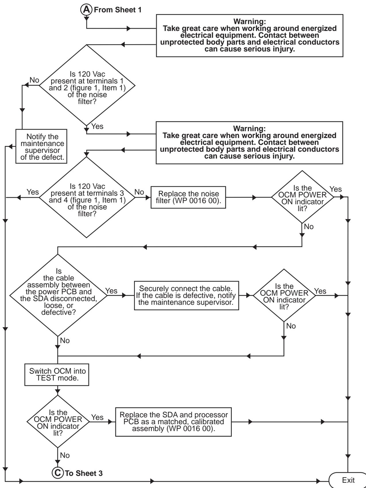
Procedure 11. OCM POWER ON Indicator Does Not Light (Sheet 2 of 3)
