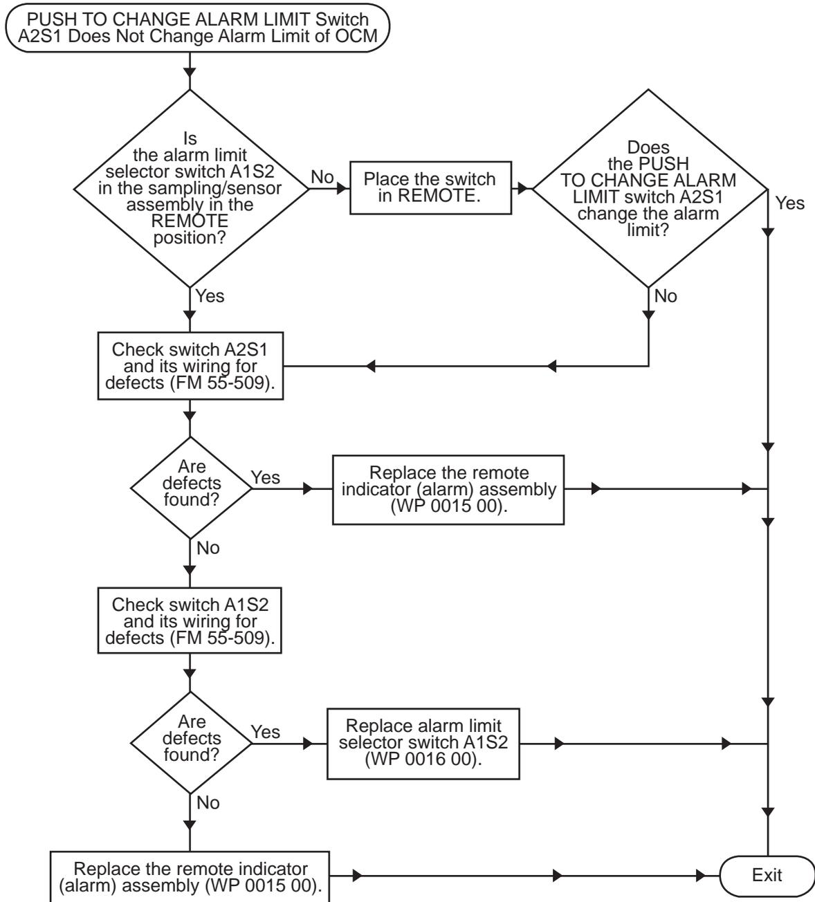
Procedure 19. PUSH TO CHANGE ALARM LIMIT Switch A2S1 Does Not Change Alarm Limit Of OCM
