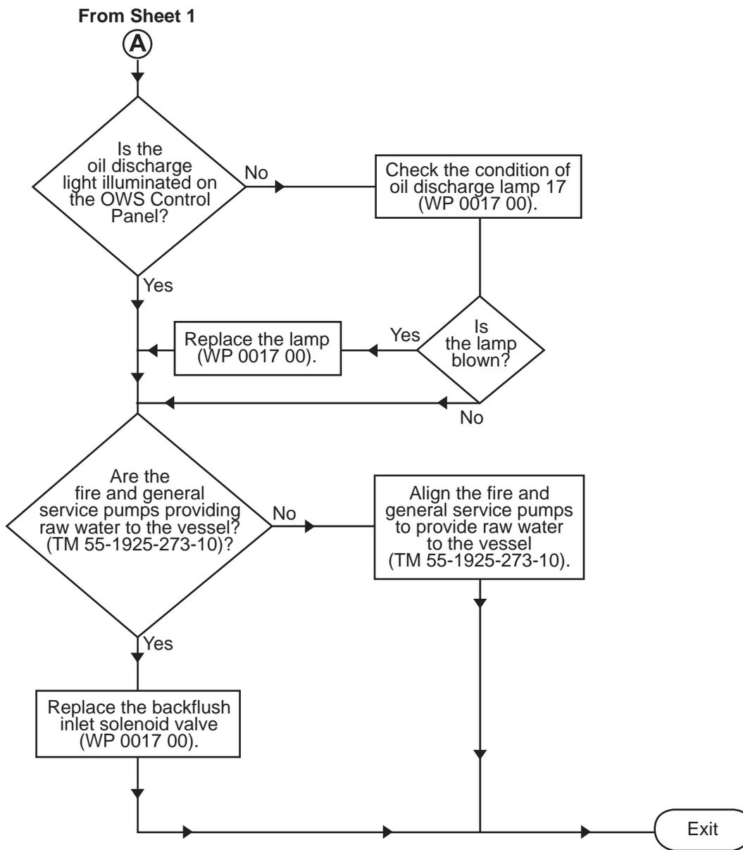
Procedure 9. Oil Does Not Discharge (Backflush) From OWS (Sheet 2 of 2)
