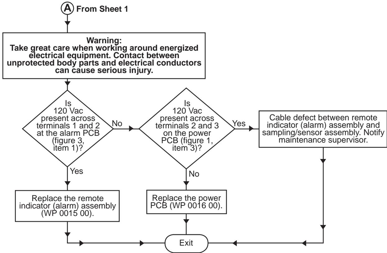
Procedure 20. Audible Alarm Inoperative when OCM Is In ALARM Mode (Sheet 2 of 2)
