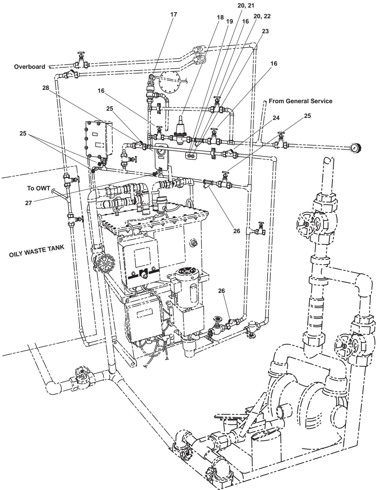
Figure 1. Oil Water Separator (Sheet 4 of 8)
