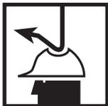
**HELMET PROTECTION** - arrow bouncing off head with helmet shows that falling parts present a danger.
