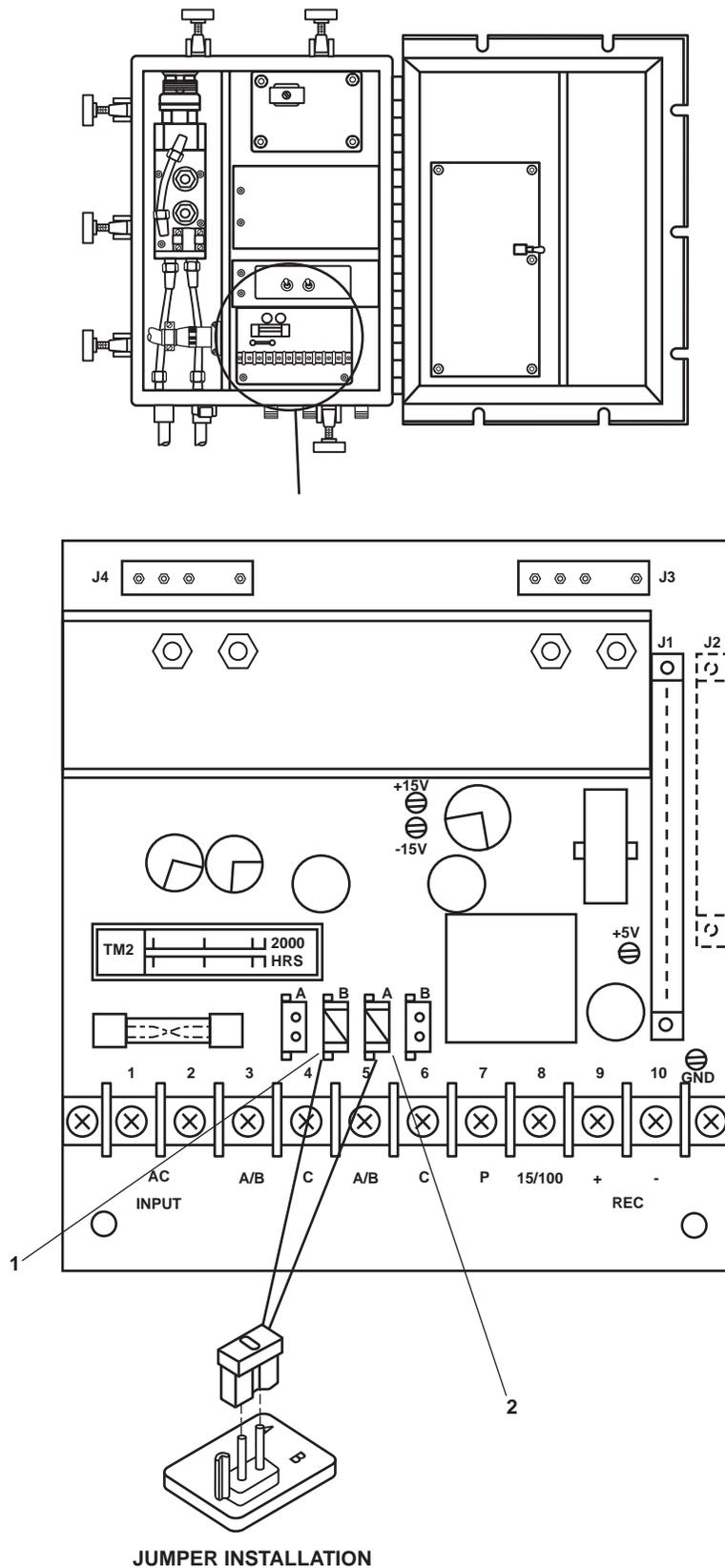
Figure 2. Sampling/Sensor Assembly, Power PCB Jumper Installation
