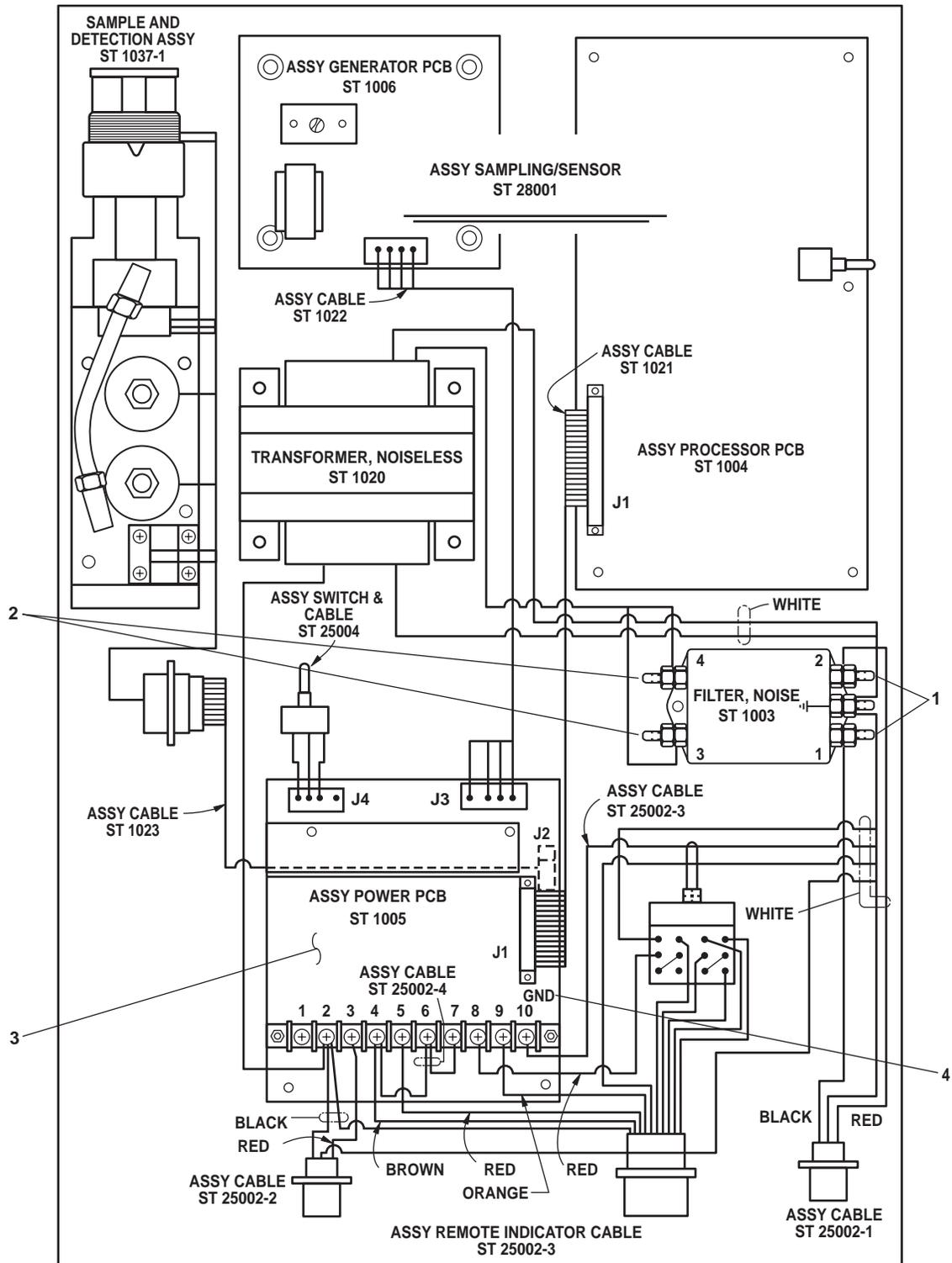
Figure 1. OCM Sampling/Sensor Assembly Wiring Diagram
