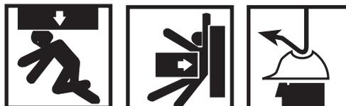
All personnel in the vicinity of the lifting operations should wear appropriate safety equipment including gloves, hard hat, and safety shoes. Death or serious injury can result from failure to heed this warning.
