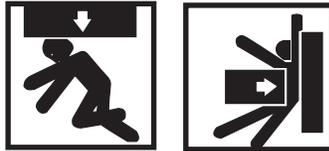
**Heavy loads can crush. Do not allow any body parts to come under the tank cover or between the tank cover and a stationary object. Death or serious injury can result.**
