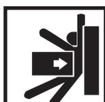
**HEAVY PARTS** - heavy object pinning human figure against wall shows that heavy, moving parts present a danger to life or limb.
