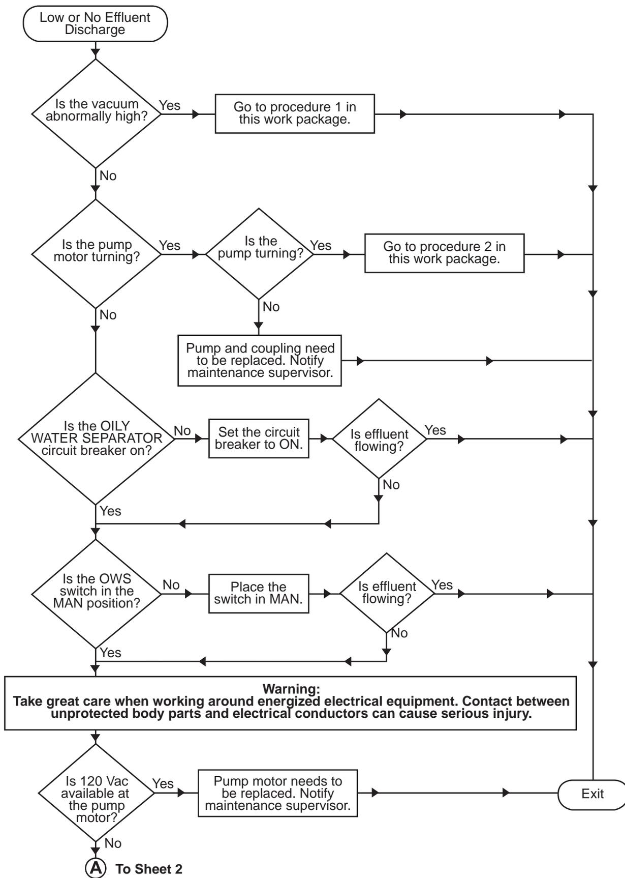
Procedure 4. Low Or No Effluent Discharge (Sheet 1 of 2)
