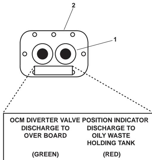
Figure 5. Diverter Valve Position Indicator
