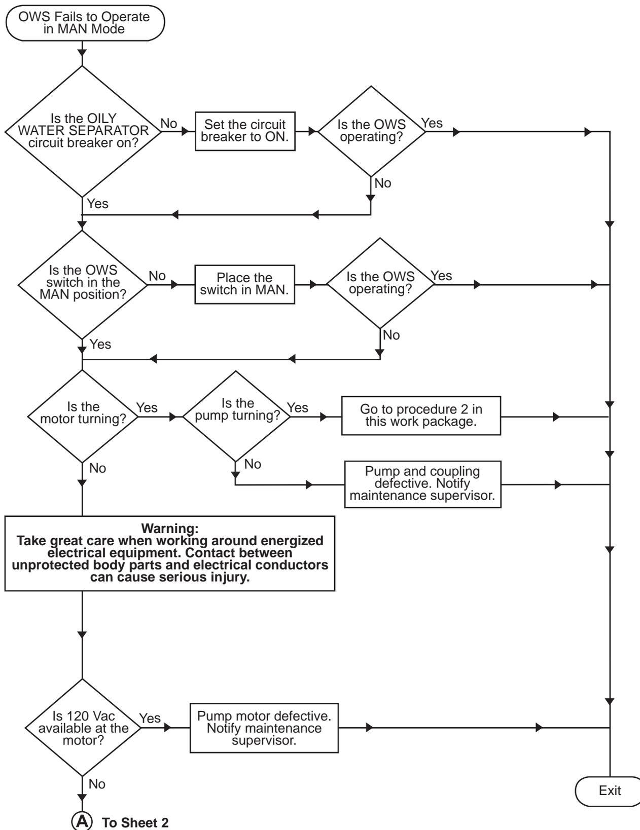
Procedure 7. OWS Fails To Operate In MAN Mode (Sheet 1 of 2)
