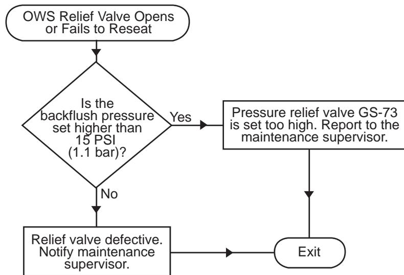
**Procedure 6. OWS Relief Valve Opens Or Fails To Reseat**
