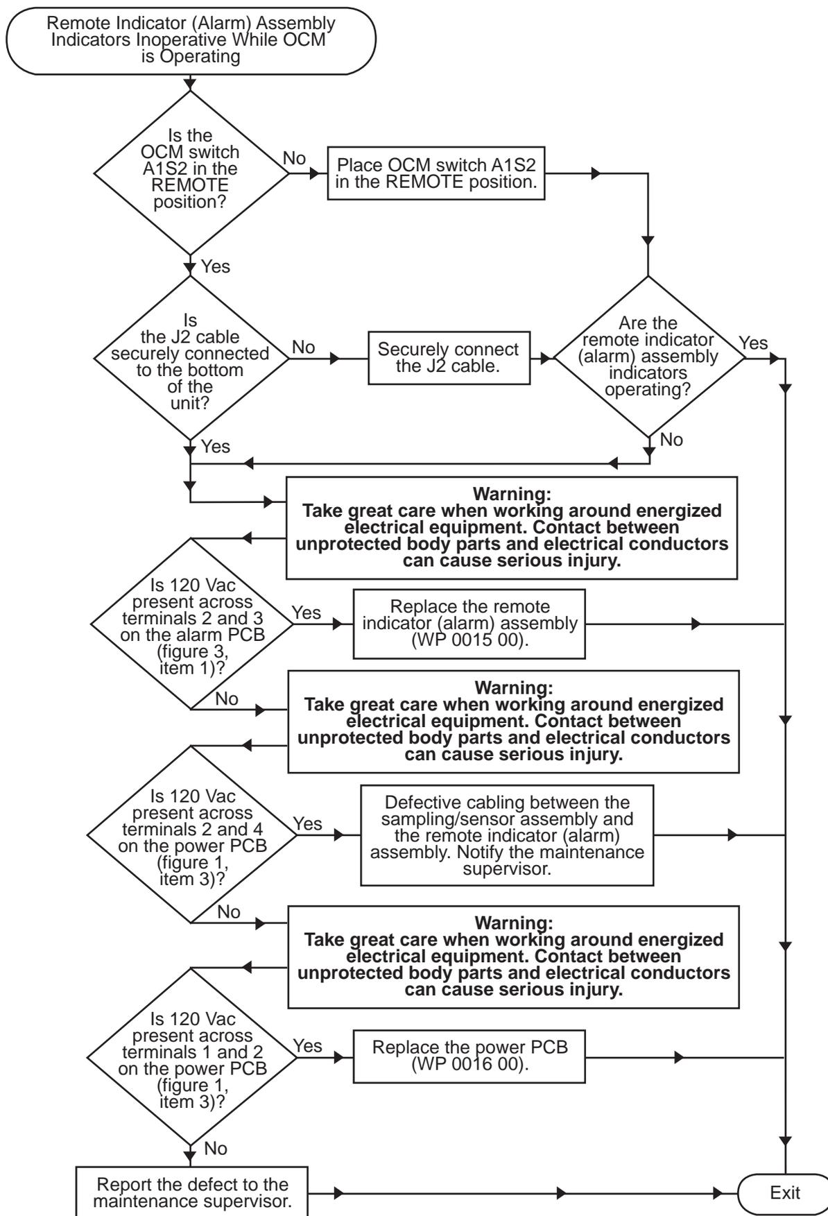
Procedure 18. Remote Indicator (Alarm) Assembly Indicators Inoperative While OCM Is Operating
